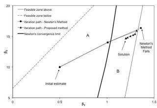
Figure 1. Iteration path for Example 4 from Okuno et al. Newton's iterations (dot) and proposed method (triangles).
