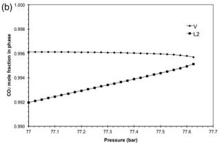
Figure 11. Phase  $CO_2$  mole fraction, vapor V (diamonds),  $CO_2$ -lean liquid  $L_1$  (triangles), and  $CO_2$ -rich liquid  $L_2$  (squares) for pressure trajectory across the three-phase envelop for  $CO_2$  mixing with Oil B at 307.6 K.
