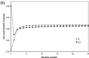
Figure 13. Convergence evolution in the outer loop for phase  $CO_2$  mole fractions, vapor V (diamonds),  $CO_2$ -lean liquid  $L_1$  (triangles), and  $CO_2$ -rich liquid  $L_2$  (squares) for  $CO_2$  mixing with Oil B to give 75% mol. of  $CO_2$  at 307.6 K and 83.5 bar.
