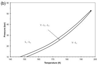
Figure 16. The phase diagram for PEMEX Gas Condensate A showing the phase regions.
