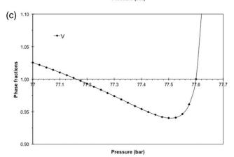
Figure 10. Phase fractions, vapor V (diamonds), CO<sub>2</sub>-lean liquid  $L_1$  (triangles), and CO<sub>2</sub>-rich liquid  $L_2$  (squares) for pressure trajectory across the three-phase envelop for CO<sub>2</sub> mixing with Oil B at 307.6 K.
