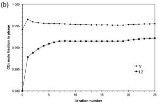
Figure 15. Convergence evolution in the outer loop for phase CO<sub>2</sub> mole fractions, vapor *V* (diamonds), CO<sub>2</sub>-lean liquid *L*<sub>1</sub> (triangles), and CO<sub>2</sub>-rich liquid *L*<sub>2</sub> (squares) for CO<sub>2</sub> mixing with Oil B to give 99.3% mol. of CO<sub>2</sub> at 307.6 K and 77.2 bar.
