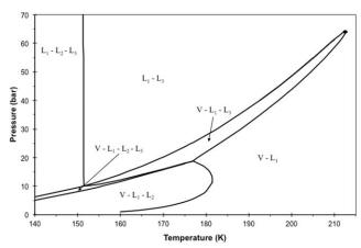
Figure 17. The phase diagram for CO<sub>2</sub> mixing with PEMEX Gas Condensate A showing the phase regions.
