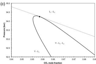
Figure 4. The phase diagram for CO<sub>2</sub> mixing with Malhamar Reservoir Oil at 305.35 K showing the phase regions.
