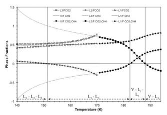
Figure 19. Phase fractions, vapor V (circles), heavy hydrocarbons-rich liquid  $L_1$  (triangles),  $CO_2$ rich liquid L2 (asterisks), CH4-rich liquid L3 (squares) for temperature trajectory across the phase diagram for CO2 mixing with PEMEX Gas Condensate A at 30 bar K.
