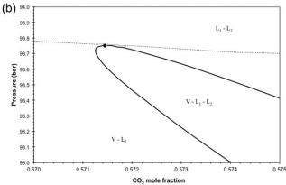
Figure 7. The phase diagram for CO₂ mixing with North Ward Estes Oil at 301.48 K showing the phase regions.
