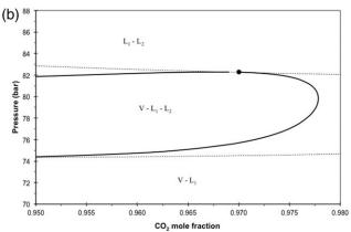
Figure 6. The phase diagram for CO<sub>2</sub> mixing with Bob Slaughter Block Oil at 313.71 K showing the phase regions.
