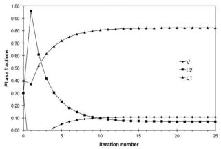
Figure 12. Convergence evolution in the outer loop for phase fractions, vapor V (diamonds),  $CO_2$ -lean liquid  $L_1$  (triangles), and  $CO_2$ -rich liquid  $L_2$  (squares) for  $CO_2$  mixing with Oil B to give 75% mol. of  $CO_2$  at 307.6 K and 83.5 bar.
