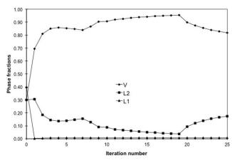
Figure 14. Convergence evolution in the outer loop for phase fractions, vapor *V* (diamonds), CO<sub>2</sub>-lean liquid *L*<sub>1</sub> (triangles), and CO<sub>2</sub>-rich liquid *L*<sub>2</sub> (squares) for CO<sub>2</sub> mixing with Oil B to give 99.3% mol. of CO<sub>2</sub> at 307.6 K and 77.2 bar.
