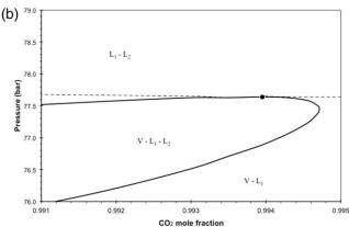
Figure 3. The phase diagram for CO<sub>2</sub> mixing with Oil B at 307.6 K showing the phase regions.
