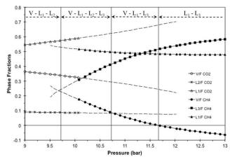
Figure 18. Phase fractions, vapor V (circles), heavy hydrocarbons-rich liquid  $L_1$  (triangles),  $CO_2$ -rich liquid  $L_2$  (asterisks),  $CH_4$ -rich liquid  $L_3$  (squares) for pressure trajectory across the phase diagram for  $CO_2$  mixing with PEMEX Gas Condensate A at 155 K.
