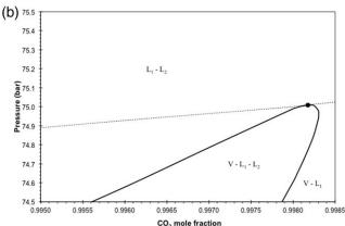
Figure 5. The phase diagram for CO<sub>2</sub> mixing with Malhamar Separator Oil at 305.35 K showing the phase regions.
