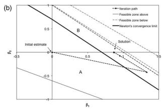
Figure 2. Iteration path for Example 3 from Okuno et al. 7 for two initial estimates.
