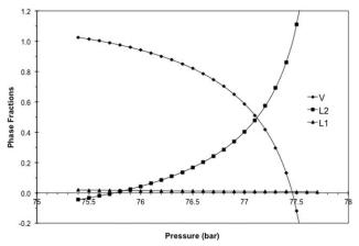
Figure 8. Phase fractions, vapor V (diamonds), CO<sub>2</sub>-lean liquid  $L_1$  (triangles), and CO<sub>2</sub>-rich liquid  $L_2$  (squares) for pressure trajectory across the three-phase envelop for CO<sub>2</sub> mixing with Oil B at 307.6 K.
