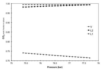
Figure 9. Phase  $CO_2$  mole fraction, vapor V (diamonds),  $CO_2$ -lean liquid  $L_1$  (triangles), and  $CO_2$ -rich liquid  $L_2$  (squares) for pressure trajectory across the three-phase envelop for  $CO_2$  mixing with Oil B at 307.6 K.
